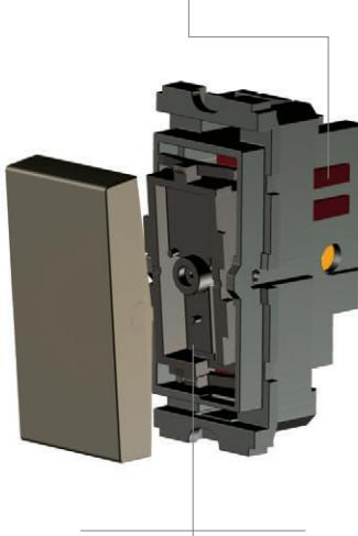
Inner shield for extra safety. It prevents the arcing from coming in contact with the front rocker. Also muffles the operating sound.
