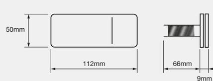
**Installation casing for in-wall applications for Round and Square Sigma Remote Buttons**
