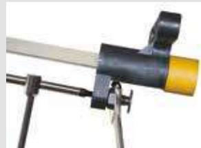
**3** - Duly adjusted, the reversible stop permits to position the rod always with a micrometric precision, in different times both on the frames and on the doors.
