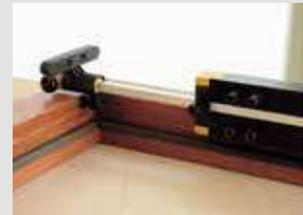
**4** - The first, easy action to drill the frame, is the correct reversible stop Positioning on the frame reference.
