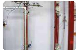
Test for resistance to wear (detail)
