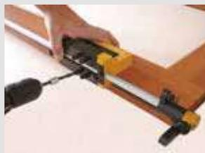
**6** - As for the door the process is the same, the correct reversible stop Positioning on the door reference, is the first operation to be done while drilling.
