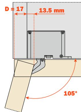
**Drilling scheme for the hinge**
